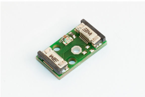
1: A member of the family: brightness sensor AS01L
